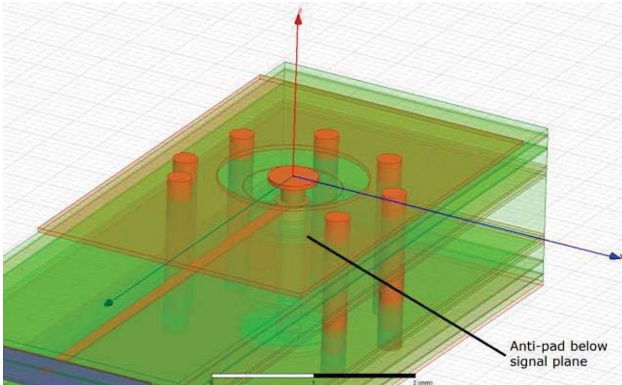
**Figure 18: Stripline Model Showing the Through 83 mil Diameter Ground Via Bolt Circle Coax Structure**
