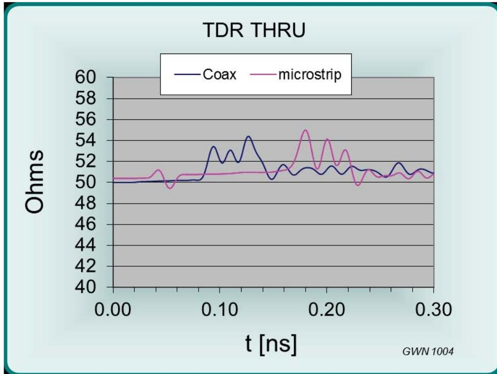
Figure 21: Optimized Time Domain Reflection Simulation (Step Response Rise Time: 10 ps)
