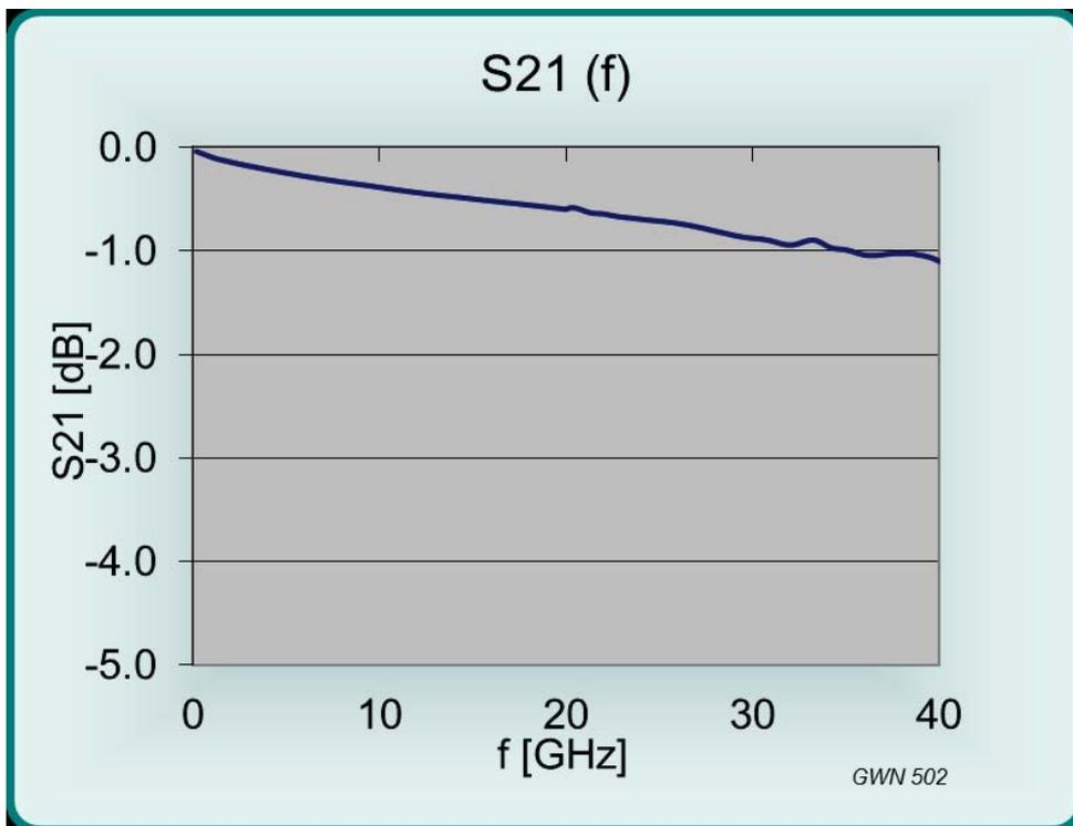
Figure 20: Optimized Insertion Loss Simulation
