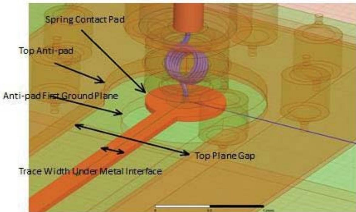
Figure 17: Tuned Simulation Parameters
