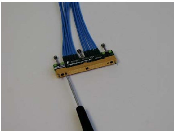
Figure 12: Removing the M1 Screws
