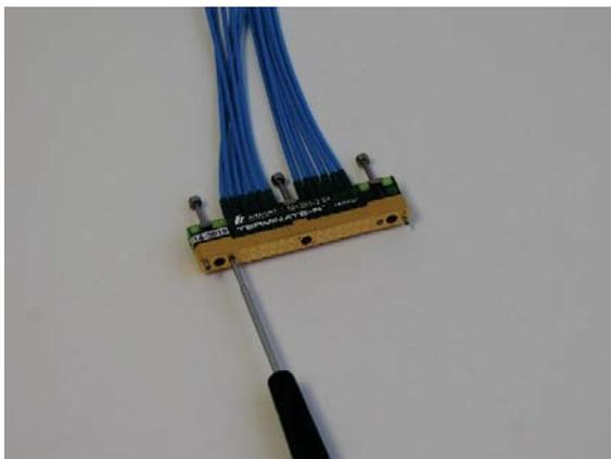
Figure 12: Removing the M1 Screws
