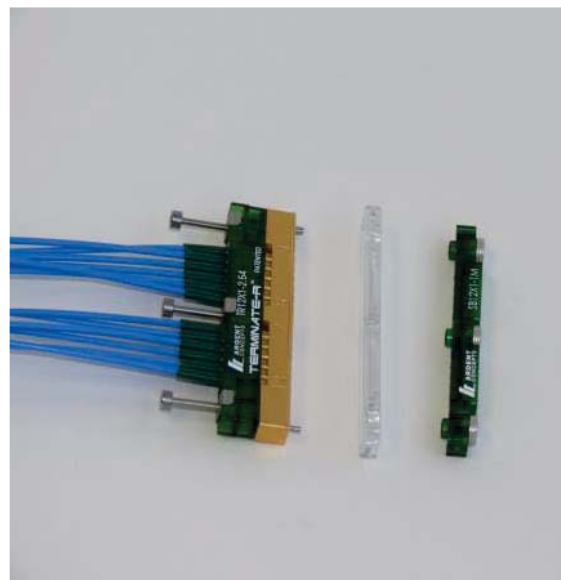
Figure 2: Protective Bottom Cover and Stiffener Block Removed from the TR Assembly
